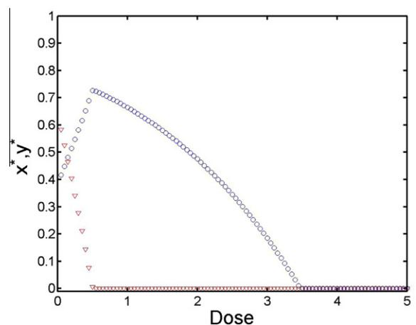
**Fig. 10.** Evolution of 20,000 initial values of  $x^*$  and  $y^*$  selected at random in the unitary square ( $0 \leq x^* \leq 1, 0 \leq y^* \leq 1$ ), for regimen II. The circles and triangles represent the values of  $y^*$  and  $x^*$ , respectively. Each initial value is iterated 10,000 but only last 1000 are shown. The parameters used are:  $a = 2, b = 1, c = 1, d = 3, e = 3, f = 1, T = 0.01, \alpha_x = 0.33, \beta_x = 0.02, \alpha_y = 0.06$  and  $\beta_y = 0.02$ .
